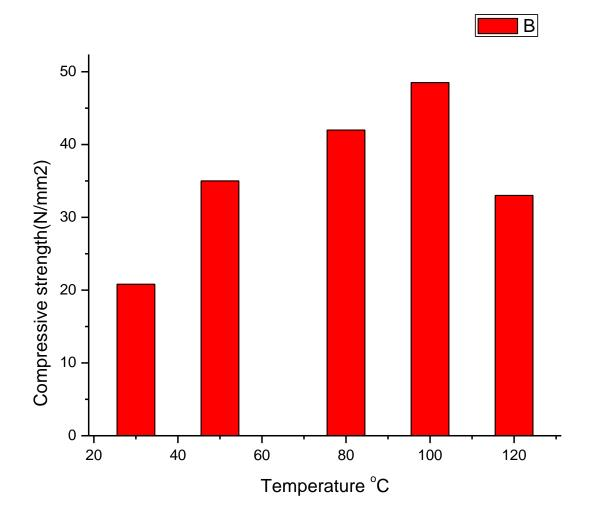
Fig1. Effect of temperatures on the compressive strength of Mix3
