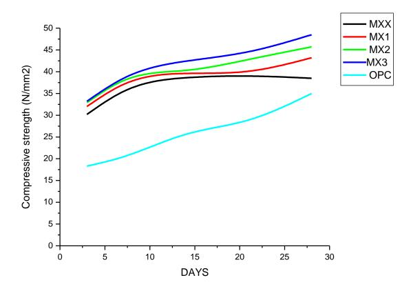
Fig.2. Compressive strength of geopolymer concrete in relation to control
