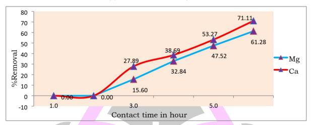
Fig.3.4 Effect of contact time on Ca and Mg ions removal using 2g cactus powder at initial 4 ppm of Ca and Mg at different time (hour).
