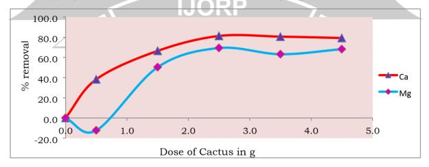
Fig.3.3.percentage removal capability of cactus powder Ca and Mg metal from hard water treatment
