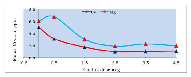
Fig.3.2.Effect of cactus dose on decrement of Ca and Mg metal from hard water at initial Concentration of 4ppm and 6ppm, respectively.
